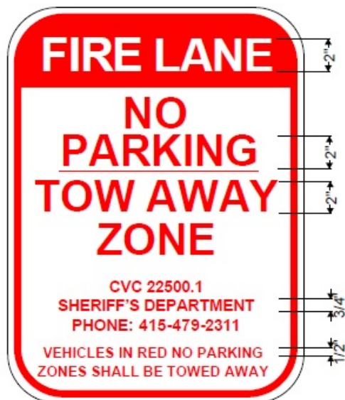
Fire Lane Sign #1 12 X 18" Red on White Reflective/Commercial Grade .080 Gauge
