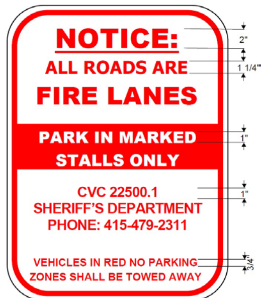
Fire Lane Sign #2 18" X 24" Red on White Reflective/Commercial Grade .080 Gauge
